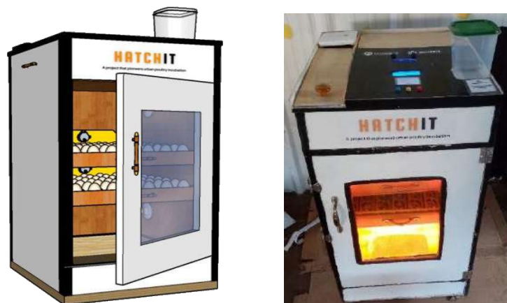
Figure. 6: HATCHIT Incubator Prototype CAD (Left) and Actual Prototype (Right)
